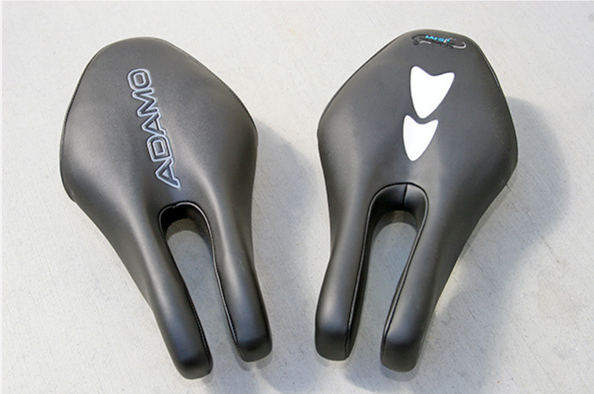
You can see the slightly more tapered nose on the ISM Adamo Time Trial (left) and the more blunt nose on the ISM Adamo Racing 2 (right).
