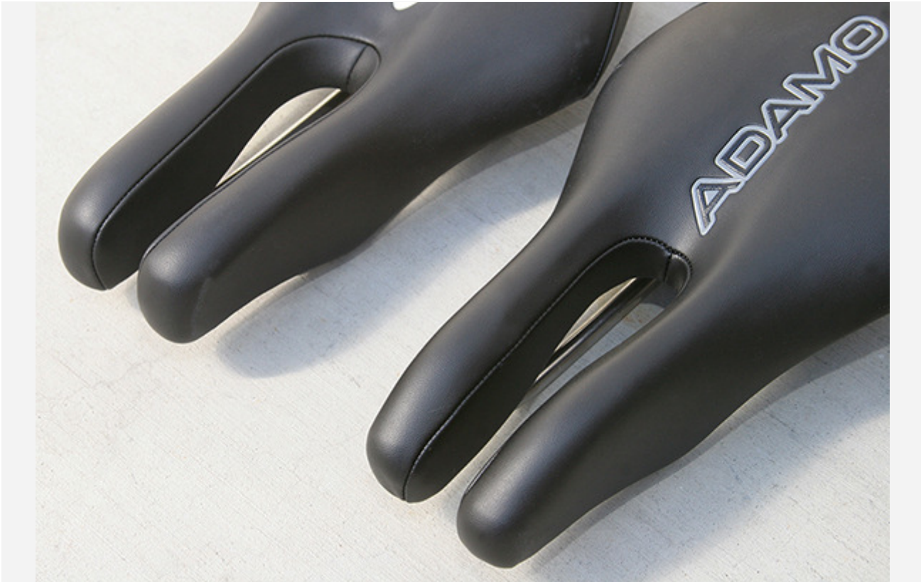
Subtle differences in the shape of the nose on the ISM Adamo Racing 2 (left) and the ISM Adamo Time Trial offer good alternatives to find the perfect fit for each rider.
