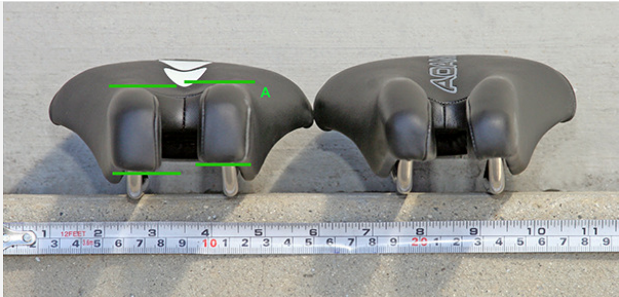
You can see the difference in the shape of the nose on the ISM Adamo Racing 2 (left) and the Time Trial. If the nose protrusions are asymmetrical they can easily be bent into place.
