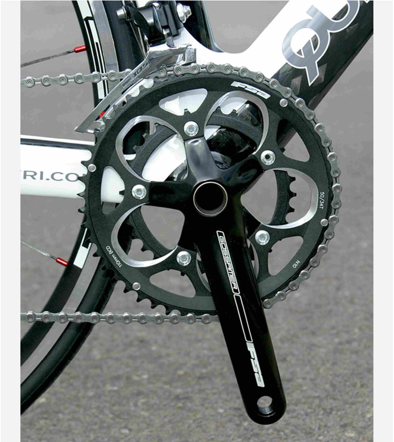
With shift pins and machined chainring your front shifting will be good between the 34 tooth small and 50 tooth large rings.
