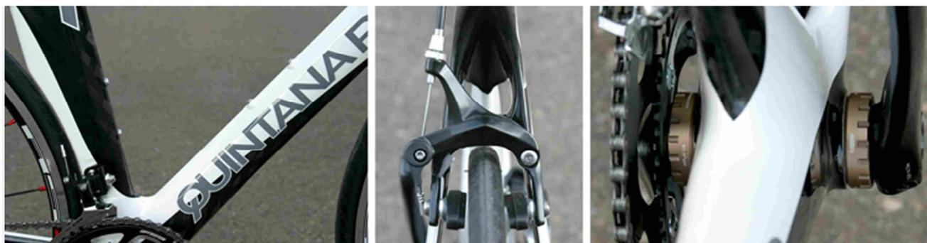
The main frame uses two conventional bottle braze ons, a strong, practical detail on an aero bike. The new rear triangle provides better ride quality. A conventional bottom bracket is easy to maintain- if it ever needed maintenance, which is unlikely.
