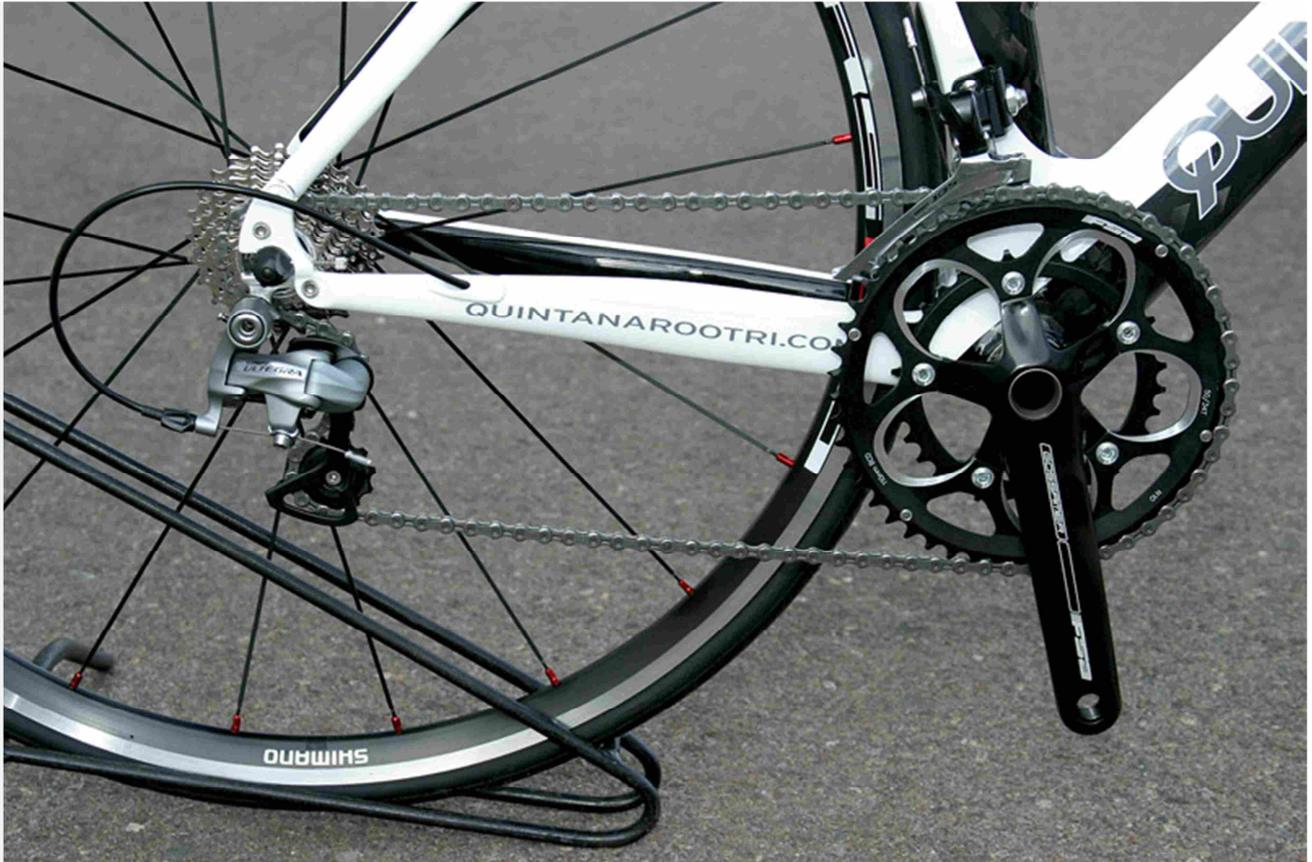
The new Shimano Ultegra rear derailleur has a wider gear capacity than previous models and great looks. A compact crank provides wider gear ratios and solid front shifting, especially from small ring to large.
