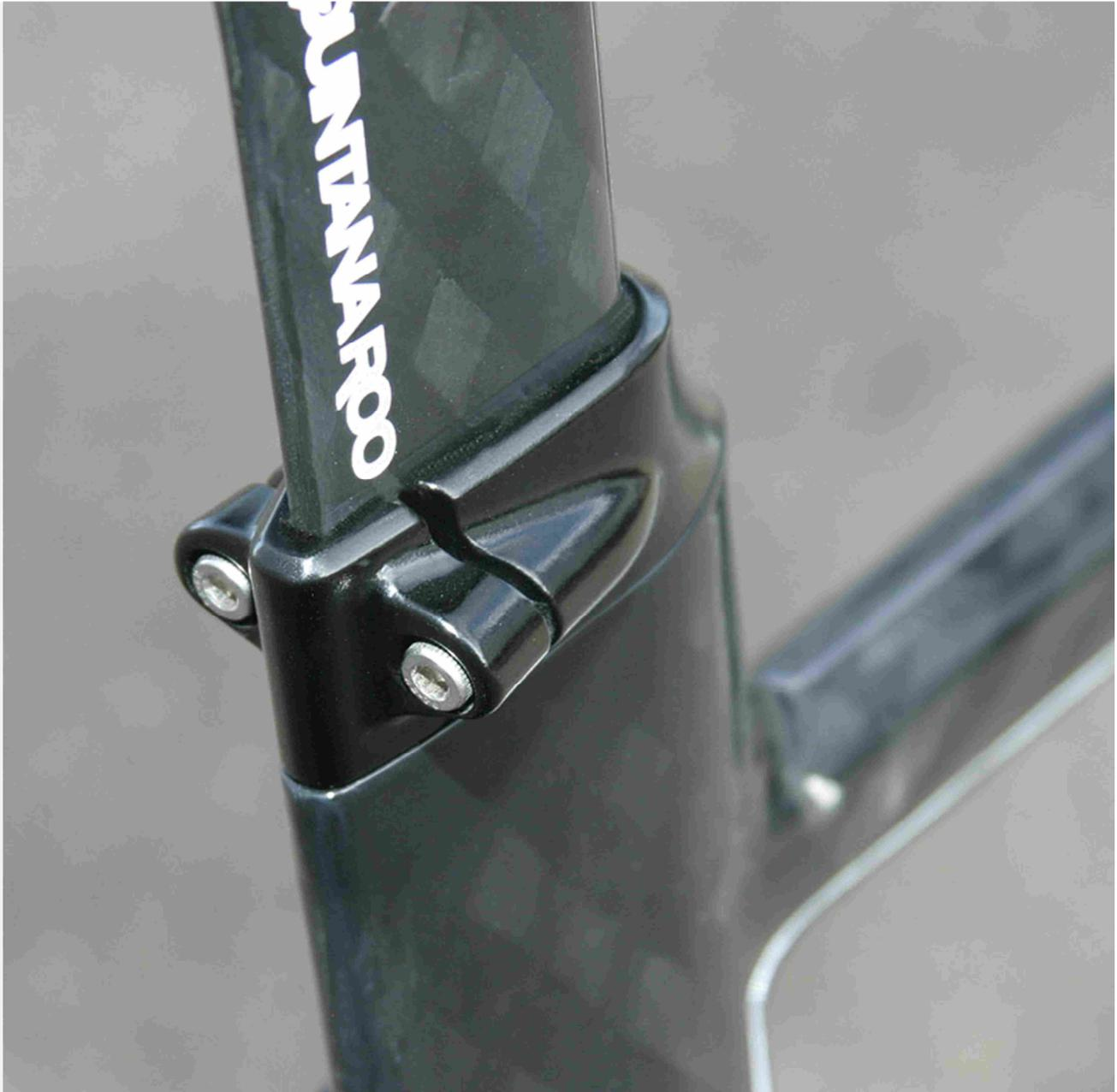
The alloy binder collar and dependable, simple seatpost binder bolts are worth a close look. This configuration is durable and dependable. Be sure you use a torque wrench and equal torque on both sides of the collar.
