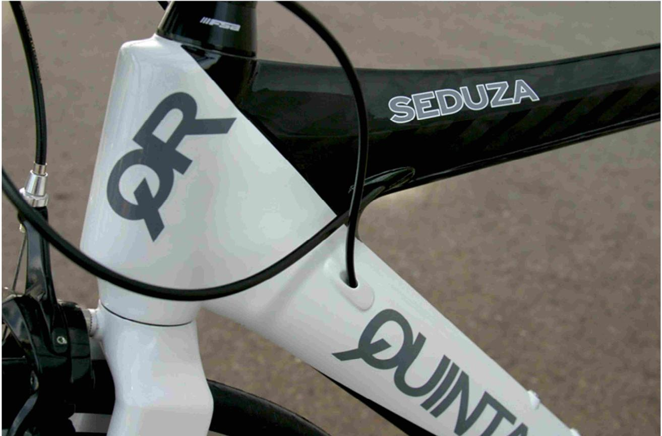
A new higher head tube on the 2011 Seduza make this bike easier to fit and more comfortable to ride. It may also make the bike faster since most riders will be able to remain in the aero position longer.
