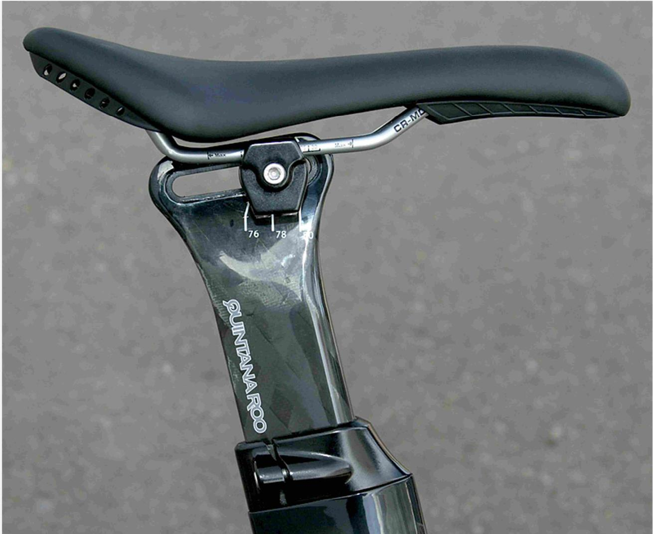
One of the strongest fit features on the Seduza is the excellent variable geometry seatpost head with infinite adjustment. It is easy to work on and reliable. The saddle specification is adequate if unremarkable.
