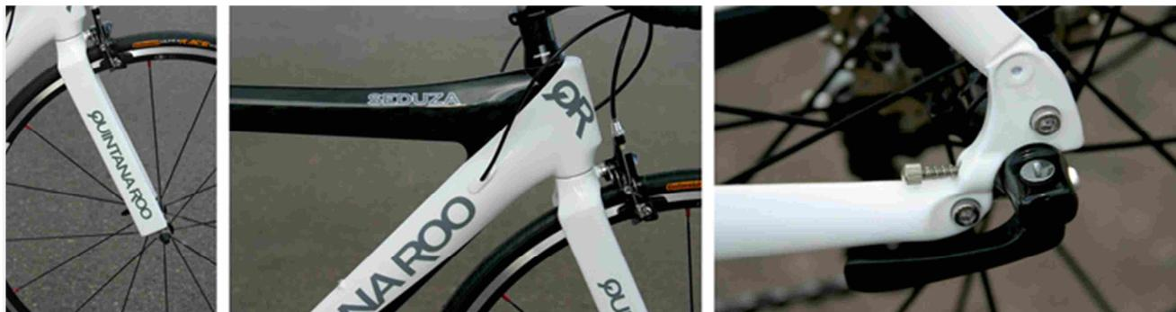
Key frame features include the Carbonaero aerodynamic carbon fiber fork, excellent, guided internal cable routing on an aero styled frame and easy to adjust drop out screws.
