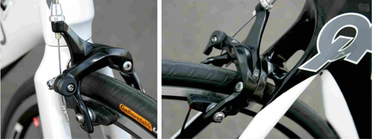
The Original Equipment Manufacturer (OEM) brakes are basic but effective. They feature an alloy barrel adjuster (not plastic) and use commonly available brake pads.
