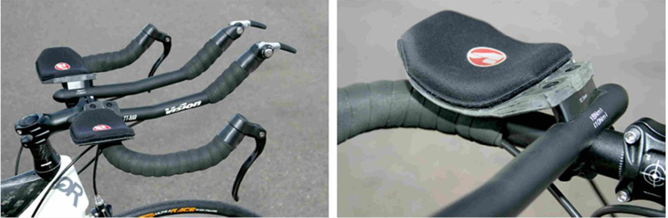
Cockpit on the 2011 Seduza uses ski bend aerobars and spring loaded brake levers with genuine Shimano Dura-Ace shifters. The stiffer elbow pads are an improvement.
