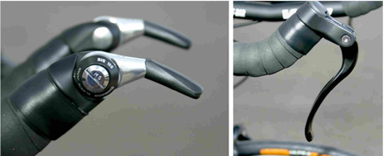
Genuine Shimano Dura-Ace bar end shifters and basic but workman-like brake levers with return springs for good actuation and return.
